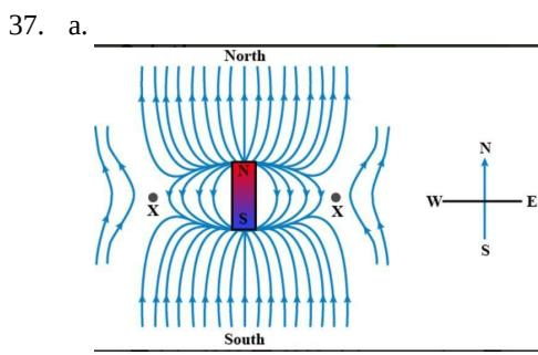
the poles are mentioned in the given figure and the magnetic field will be stronger at the end of the pole.
