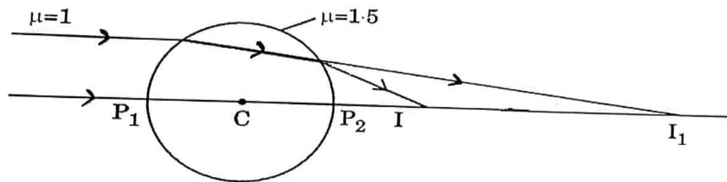
From  $I^{\text{st}}$  surface, Refraction is from rarer to denser medium and object is at  $\infty$
