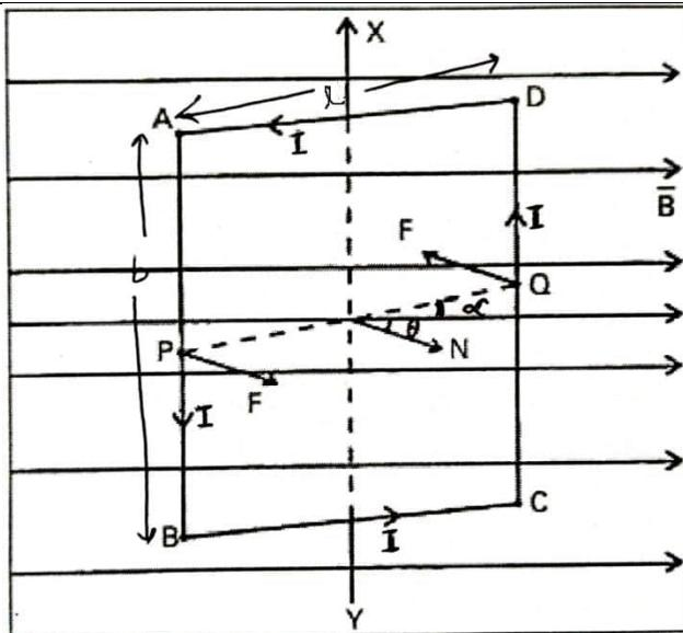
If the plane of the current carrying coil makes an angle  $\alpha$  with the magnetic field
