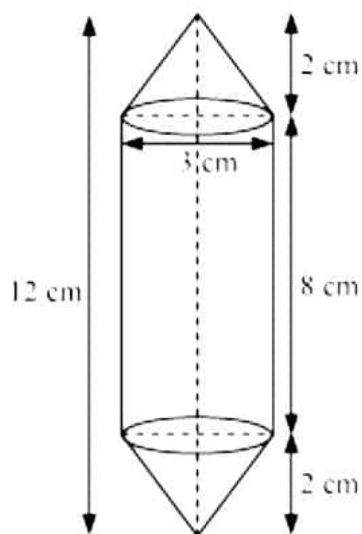
From the figure Height ( $h_1$ ) of each conical part = 2 cm
