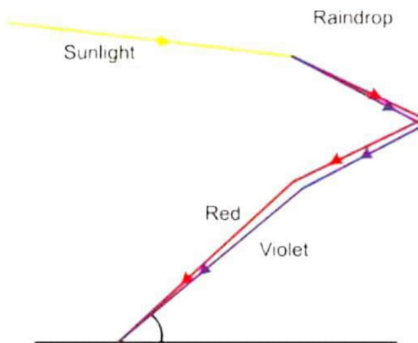
Rainbow is caused due to dispersion of sunlight by raindrops suspended in air. Water drops act like tiny prisms. Water drops refract the sunlight, disperse, then reflect internally and then refract it again. This is how a rainbow is formed.
