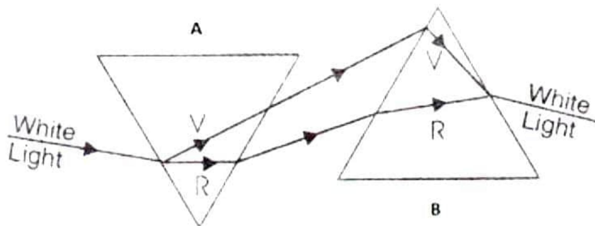
This reverse refraction occurs due to the refracting sides being parallel to each other.
