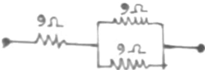
If we connected two 9 ohm resistors in parallel and other 9 ohm resistor in series as shown in figure:
