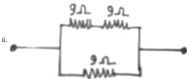
If we connected two 9 ohm resistors in series and other 9 ohm resistor in parallel as shown in figure:
