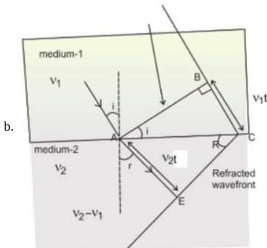
The ratio of the speed of light in vacuum to the speed of light in the medium is termed as refractive index of medium.
