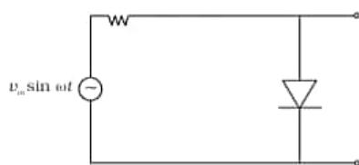
a) would be like a half-wave rectifier with negative cycles in output
