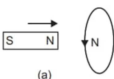
Similarly when north pole of the magnet is moved away from the coil, the direction of current in the coil will be such as to attract
