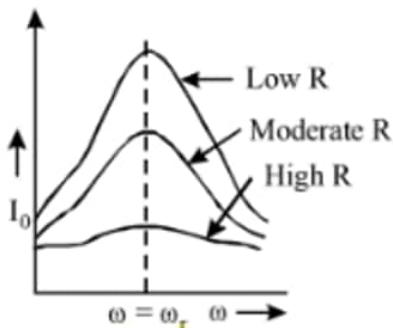
The Q-factor of the series resonant circuit is defined as the ratio of the voltage developed across the capacitance or inductance at resonance to the impressed voltage which is the voltage applied.
