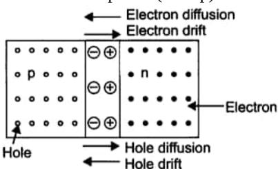
ii. **Drift:** The drift of charge carriers occurs due to electric field. Due to build in potential barrier, an electric field directed from n-region to p-region is developed across the junction. This field causes motion of electrons on p-side of the junction to n-side and motion of holes on n-side of junction to p-side. Thus a drift current starts. This current Depletion is opposite to the
