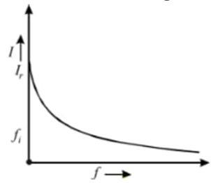
With the increase of frequency of AC source, inductive reactance increase as
