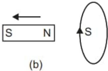
Thus, in each case whenever there is a relative motion between a coil and the magnet, a force begins to act which opposes the relative motion. Therefore to maintain the relative motion, a mechanical work must be done. This work appears in the form of electric energy of coil. Thus Lenz's law is based on conservation of energy.
