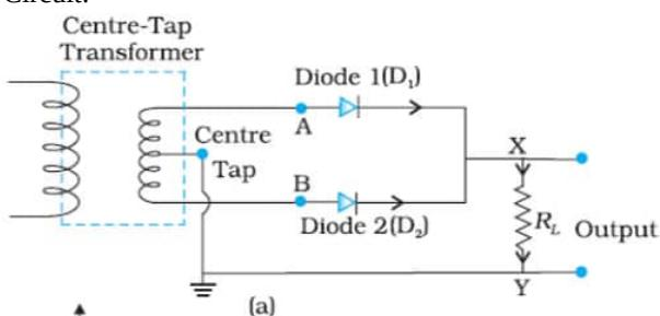
Principle:- Diode conducts only in forward biasing.
