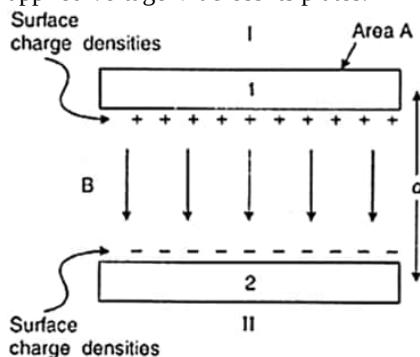
Electric field between the plates of capacitor
