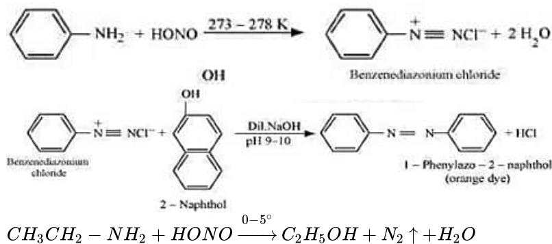
iv. Aniline and benzylamine can be distinguished by their reactions with the help of nitrous acid, which is prepared in situ from a mineral acid and sodium nitrite. Benzylamine reacts with nitrous acid to form unstable diazonium salt, which in turn gives alcohol with the evolution of nitrogen gas.
