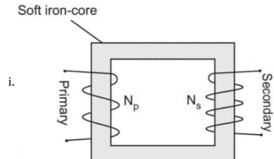
The working principle of transformer is mutual induction.
