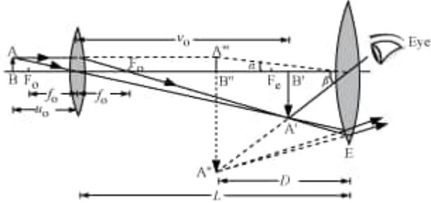
Distance between the objective and the eyepiece,  $L = v_0 + |u_e|$
