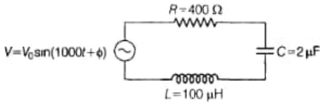
ii. Calculate the value of additional capacitor which may be joined suitably to the capacitor  $C$  that would make the power factor of the circuit unity.
