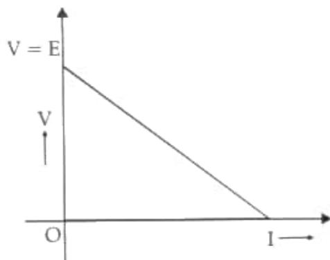
$$I = \frac{E}{R+r} \quad (\text{V} = E - Ir \text{ and } V = IR)$$
