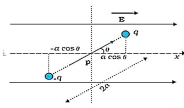
The amount of work done in rotating the dipole from  $\theta = \theta_0$  to  $\theta = \theta_1$  by the external torque
