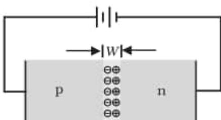
The applied voltage mostly drops across the depletion region and the voltage drop across the p-side and n-side of the junction is negligible. (This is because the resistance of the depletion region – a region where there are no charges – is very high compared to the resistance of n-side and p-side.) The direction of the applied voltage ( $V$ ) is opposite to the built-in potential  $V_0$ . As a result, the depletion layer width decreases [Fig.]
