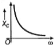
iv. For a capacitor fed with an AC supply,
