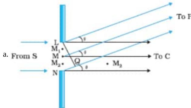
From diagram path difference between the waves from L and N =  $a \sin \theta$
