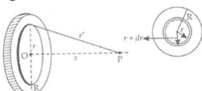
Now consider a ring of radius r of thickness dr on a disc of radius R, as shown in the figure. Let us consider disc is divided into a large number of rings. Again let the charge on the ring is dq then potential dV due to ring at P, will be
